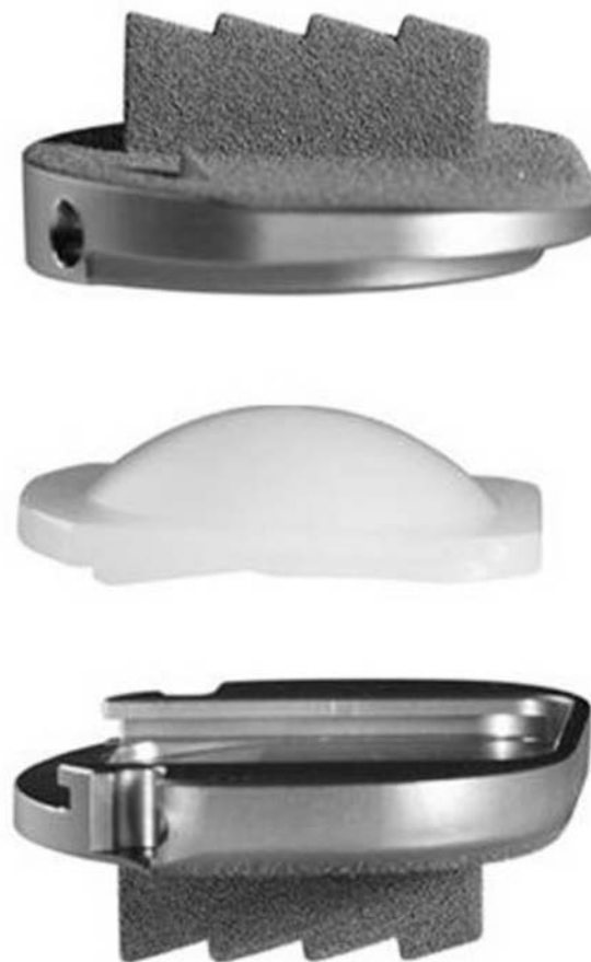
Figure 2. ProDisc artificial disc consisting of two cobalt chrome alloy endplates and a polyethylene core that is attached to the caudal endplate. The endplates have central anchoring keels that provide greater immediate fixation and are covered with a pure titanium plasmapore surface.
