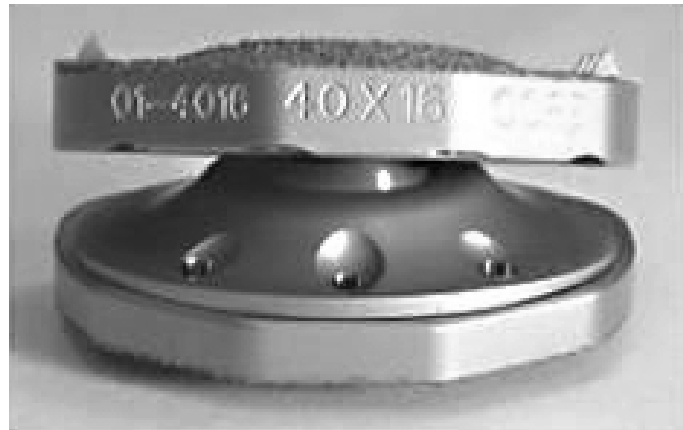
Figure 4. FlexiCore artificial disc. The design is similar to the Maverick metal-on-metal design, but the FlexiCore disc has a fixed center of rotation. Shaped endplates have small spikes and surface coating for bone ingrowth into the metal, which supplements fixation to the endplate.
